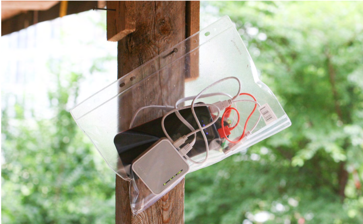
Figure 21: The hardware-setup of the first prototype: A battery pack, a Raspberry Pi and a Wi-Fi router. The compact setup was helpful in demonstrating the versatility of this technological approach to setting up DIY networks
