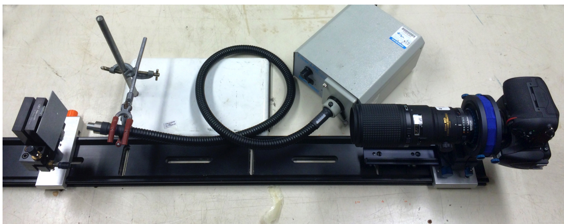
Figure 3: Image of experimental setup, visible is the Nikon D810 colour camera, macro bellows, Nikon 200mm f4 macro lens, light box, fibre optic light guide and rotation stage with target.
