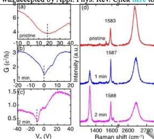
Figure 5. [(a)–(c)]  $G_{ds}$ – $V_g$  curves of the same exfoliated graphene at different doping states measured at 10 K. The dashed lines indicate the gate voltage at the charge neutrality point. (d) Raman spectra correspond to the graphene at different doping states shown in [(a)–(c)].<sup>68</sup> Reprinted with permission from Lin et al., Appl. Phys. Lett. 96, 133110 (2010). Copyright 2010 AIP Publishing LLC.
