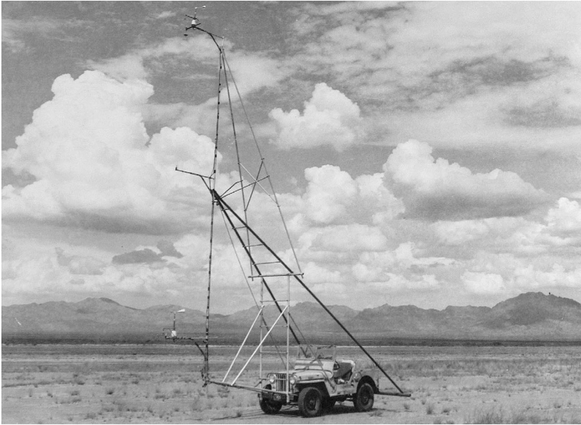
Fig. 9 Arizona desert west of Tucson, with Peter Sinclair's mobile meteorology tower mounted on the surplus jeep he used to penetrate dust devils (from Sinclair's Ph.D. thesis)
