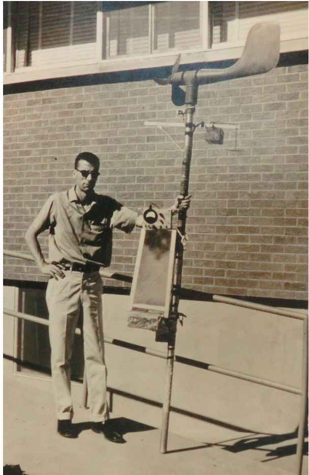
Fig. 8 Peter Sinclair with his portable measurement station with rather prominent anemometer and wind vane (from his Ph.D. thesis). The box with electrical dial is a sensitive microbarometer designed by Sinclair
