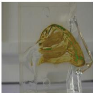
60° and 5 mm inserted 1 cm 2 in the nasal vestibule 0.9 cm 2 in middle-upper turbinates 0.6 cm 2 olfactory
