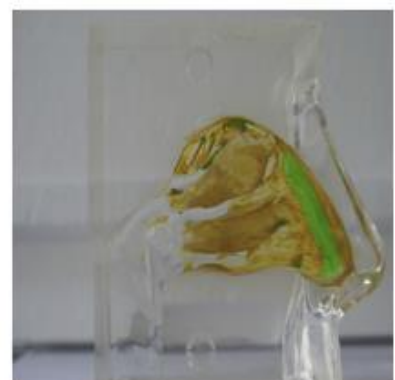
80° and 15° angled 1.35 cm 2 in nasal vestibule 4.05 cm 2 in middle-upper turbinates 0.4 cm 2 olfactory
