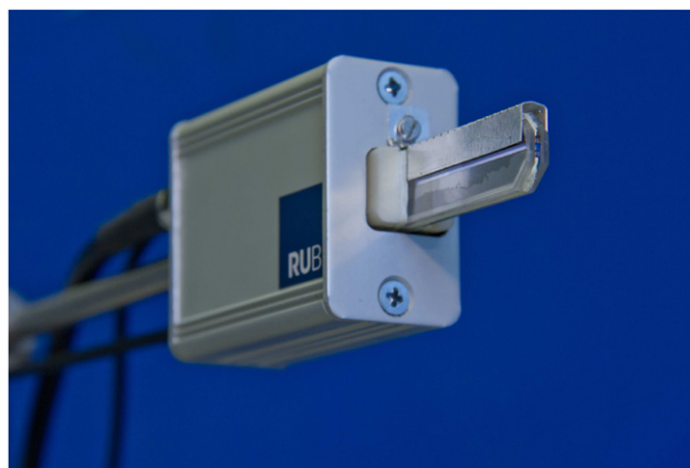
Figure 1. Photograph of the ignited COST Reference Microplasma Jet (COST-Jet). The homogeneous discharge is formed between the plane-parallel electrodes of the electrode assembly that extends from the housing.
