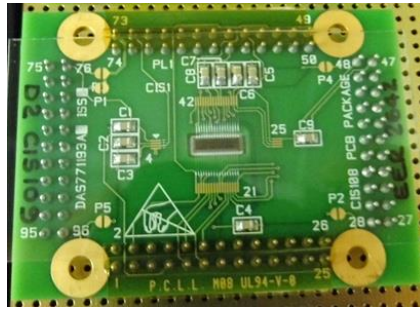
Figure 5. Photograph of CIS109 in a printed circuit board carrier.
