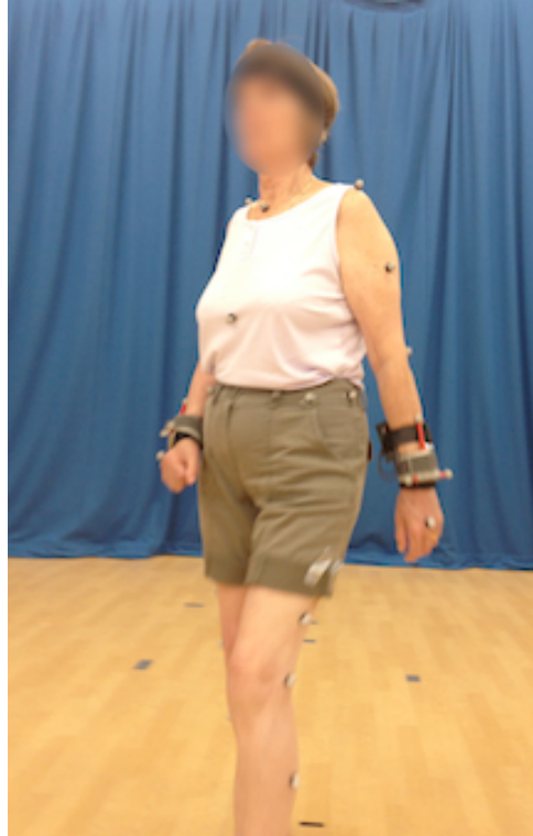
Figure 3. Tactile cued walking of a stroke survivor. As well as wearing a haptic bracelet on the paretic (right arm), the participant is wearing optical markers on the body for motion tracking.
