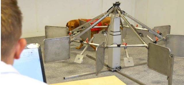
Figure 1. Carousel. The samples are suspended between metal screens preventing volatiles from traveling between positions.
