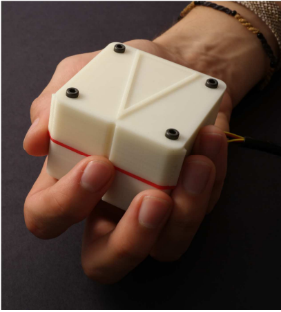
Fig 2: The Haptic Sandwich device held in hand
