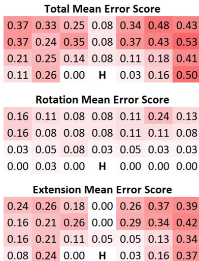
Fig 8: Average Euclidean error score per pose. Cell arrangement corresponds to the pose chart (Fig 6)
