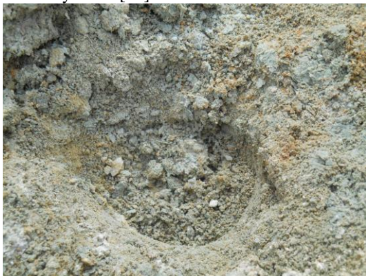
Fig. 2. Sampling location for core samples, after taking core 12, diameter of core 5 cm.
