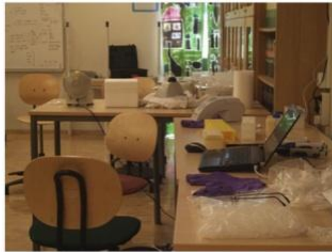
Figure 7 - The three workstations as set up in our field laboratory. (l) DNA extraction, purification, and qPCR area, with general supply table in foreground. (c) ATP bioluminescence area, with FM staining area in the background. (r) 'Darkroom' established for fluorescence microscopy.
