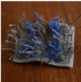
Figure 3: Rug-like swatch with conductive thread.
