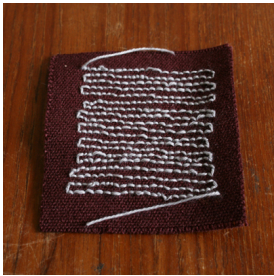
Figure 2: Needle punched swatch with conductive yarn.
