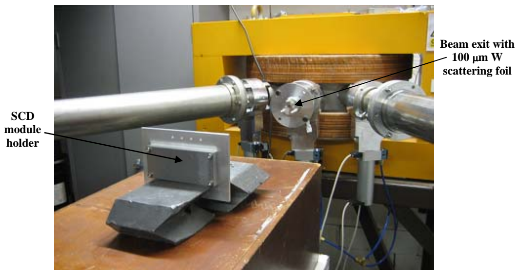
Figure 6.7: SCD mounted in line with the proton beam
