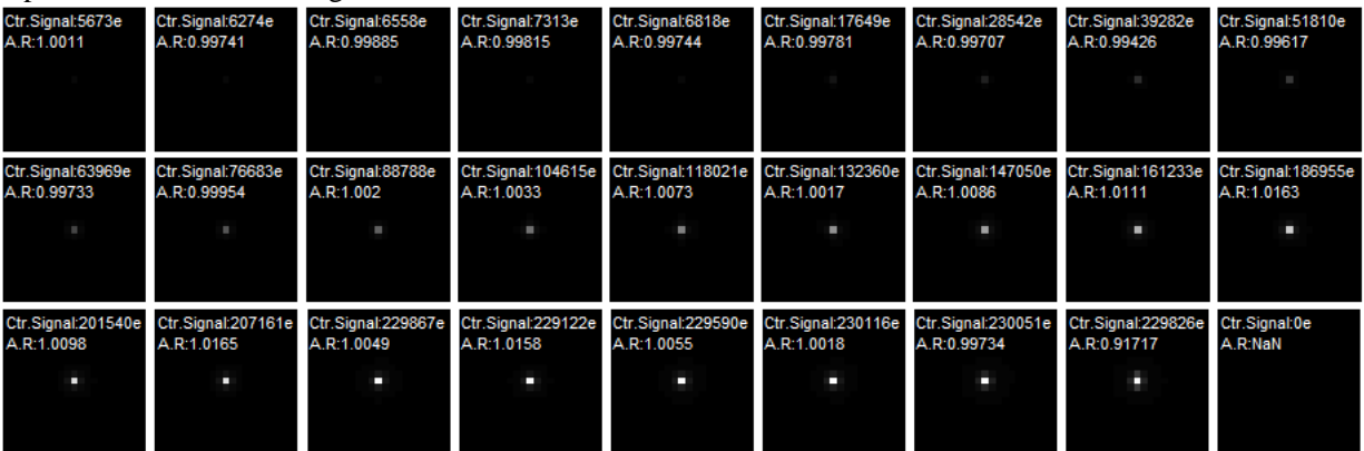
Figure 5. Two spot-plots generated from the same set of SP-PTC data. The centroiding algorithm generates average images from well-centred spots only allowing charge spreading behaviour with respect to signal to be better observed.
