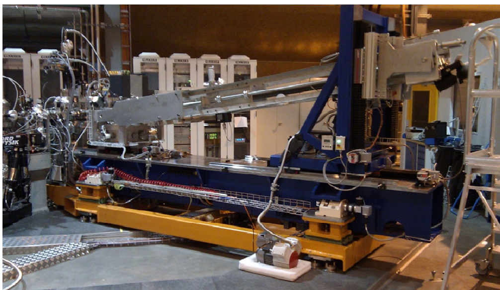
Figure 5. A photograph of SAXES, showing the main arm housing the grating (mid-left) and the black casing surrounding the detector, placed at 20° to the incident beam (upper-right). The detector system is currently based around a CCD camera.
