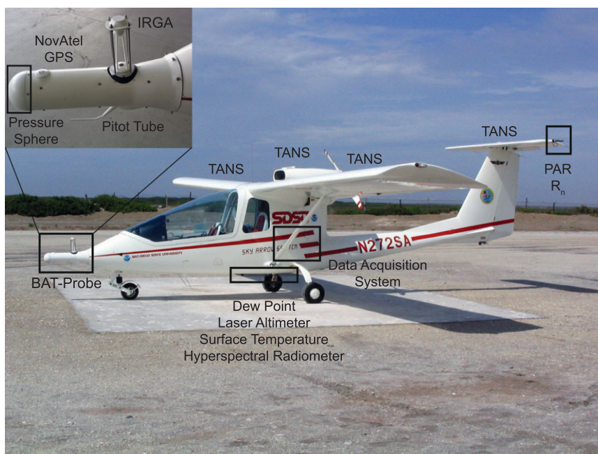
FIG. 2. Photograph of the SDSU Sky Arrow 650TCN ERA while parked at the Lopez Mateos airstrip. Locations of the sensors are shown. The BAT probe (inset) is on the nose of the aircraft while the four TANS Vector attitude GPS antennas are located on the center of each wing, top of the engine cowling, and top of the horizontal stabilizer. The data acquisition system and computers are located behind the rear seat. Downward-looking sensors are located in the two view ports in the bottom of the fuselage of the aircraft.
