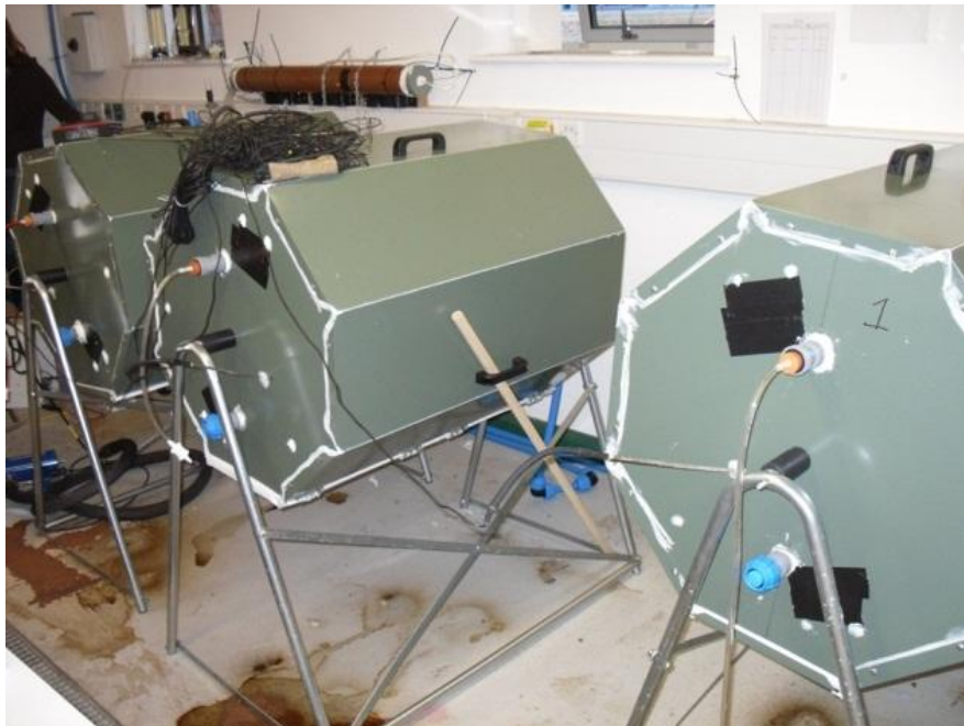
Figure 6. Composting units used for odour production.
