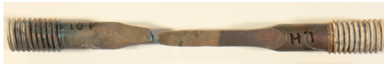
Fig. 6 The ruptured tensile specimen tested at 545°C.
