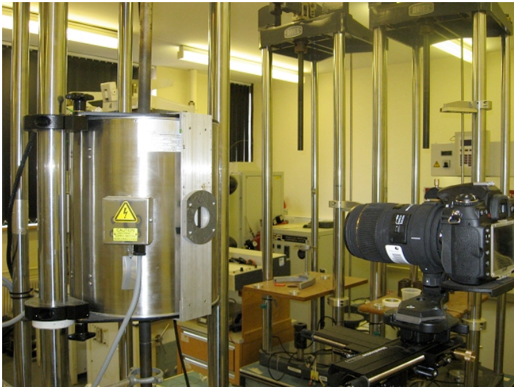
Fig. 4 DIC high temperature creep measurement system
