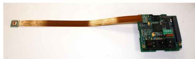
Fig. 5. Demonstration of the C3D payload controller with an e2v EV76C560 CMOS imaging sensor on a 30cm flexi
