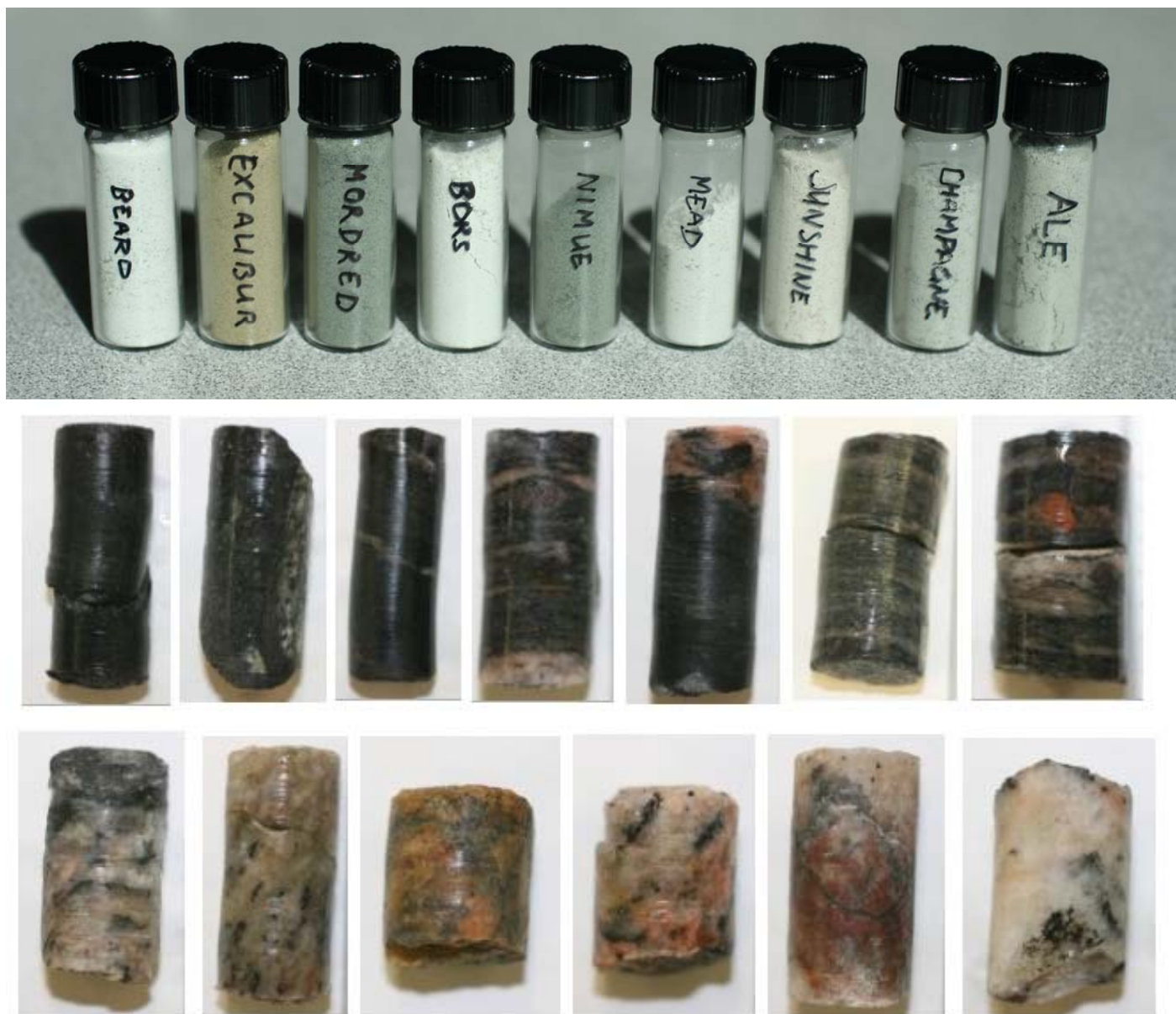
Figure 8 – (TOP) nine of the ten samples chosen by the Science Team to return to Earth, shown in powdered form. So many samples were achieved (18 total) that returning them all would not have been realistic, thus a triage was performed on the 9 th day of the deployment. (BELOW) A visual inspection of the raw cores reveals a significant variety of sampled materials with colours ranging from black to white with reddish colours also present. Note that the raw cores do not correspond to the powdered cores shown above.
