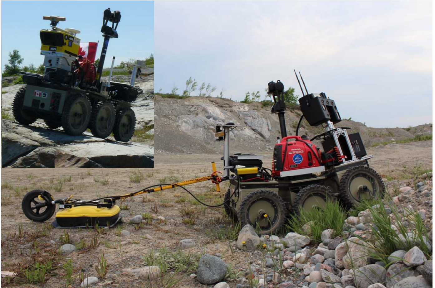
Figure 2 – The ROC-6 Rover showing instrumentation configurations. (MAIN) The gigapan camera mount is shown on a mast above the middle rover segment with the MDA C2SM camera head shown on the rightmost segment and the GPR to the left of the leftmost rover segment. In the background the “Guinevere” outcrop (See fig. 10) can be seen. This terrain is typical of the site. (INSET) During the second week the C2SM was replaced with an ILRIS LiDAR, shown in yellow, and the GPR was removed.
