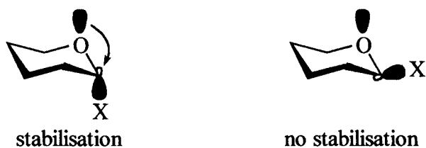
Figure 3 : Orbital interactions giving rise to the anomeric effect
