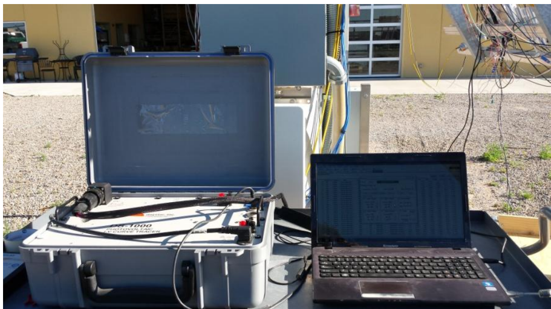
Figure 31: Daystar DS-1000 I-V curve tracer connected to a laptop.
