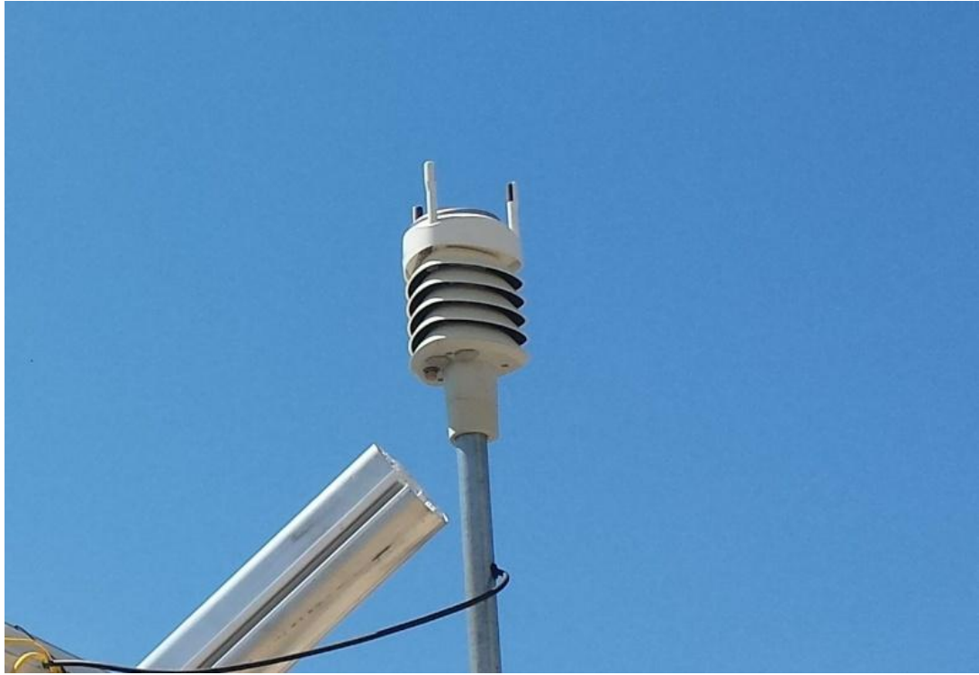
Figure 29: The Vaisala weather transmitter WXT520.
