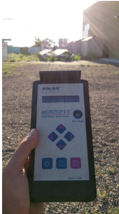
Figure 32: Solar Light Microtops II sunphotometer positioned towards the sun.
