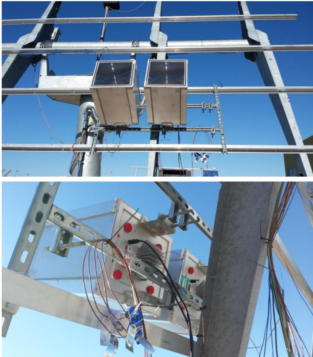
Figure 28: Front (top Figure) and rear (bottom Figure) photographs of two DDM-1090× receiver assemblies (RAs or monomodules) mounted on a high-accuracy solar tracker in Albuquerque, NM.
