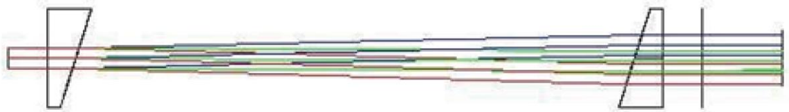
Fig. 4.4 A 'straight through' optical layout using a pair of grisms.
