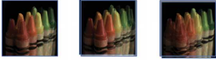
Figure 2.9: Shift and integration process (Ref. [59], Fig. 4.2) implies that a sub-aperture image (left) is overlaid with another (middle) and shifted whilst blending pixel values. The shift variation moves the synthetic focus from red crayons in the foreground (middle) to green crayons in the background (right).
