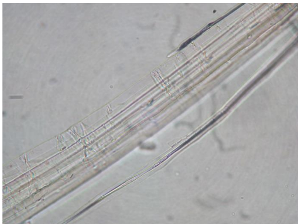
Figure 1: Jute fibre at showing cross marks and longitudinal striations (image width ~ 144 \mu\text{m} )
