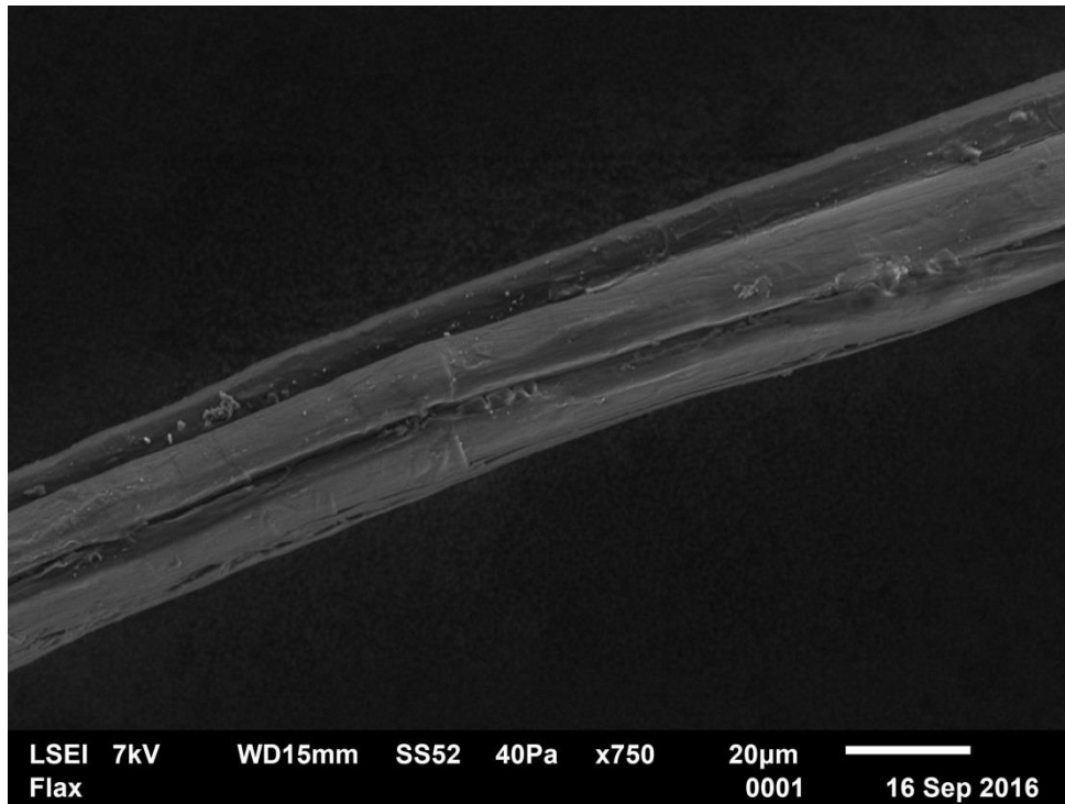
Figure 7: SEM micrograph of flax fibre
