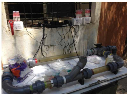
Figure 2 | Swirl Flow Bioreactor set up in the field study at The Sewage Treatment Plant, Rajiv Gandhi Infotech Park, Hinjewadi, Pune, Maharashtra, India.
