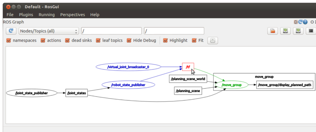
Figure 4.1: Snapshots of the rqt_graph application, a tool to visualize the ROS network. The Figure is available from http://wiki.ros.org/rqt_graph
