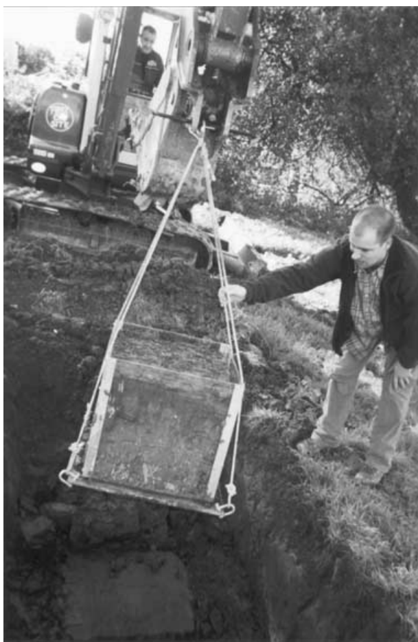
Figure 1. Extraction of an isolated soil block.
