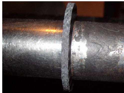
Figure 4. Transverse loading configuration without using smaller contact area
