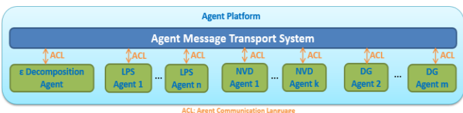
Fig. 1. MAS for optimal distributed voltage regulation within Presage2.
