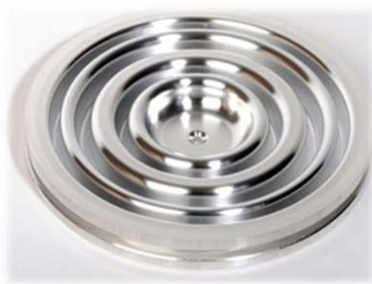
FIG. 2. The three-choked 7.8 GHz Al test cavity.
