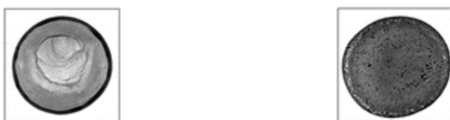
Figure 28: Dried droplets highly affected by surface tension flows (left) and unaffected by surface tension flows (right) Reprinted with permission from (Anyfantakis, Manos et al (2015) Modulation of the Coffee-Ring Effect in Particle/Surfactant Mixtures: the Importance of Particle–Interface Interactions, 31: 4113-4120). Copyright (2015) American Chemical Society.
