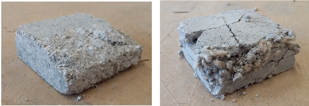
(a) Example of Incorrect Failure (IF) in sample D-W0C10-1. Note the diagonal failure across the front right corner of the image and the lack of other failure in the rest of the sample.
