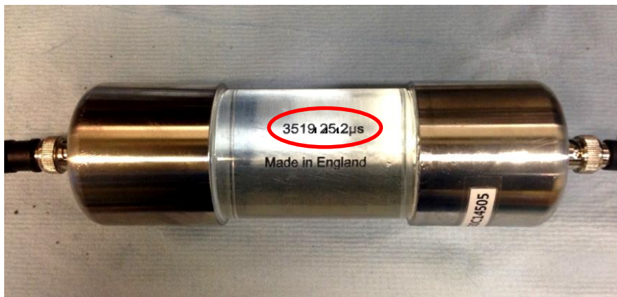
Figure 4.14: A Plexiglas calibration and receiver block with 25.2 \mu\text{s} transit time sandwiched by two piezocomposite transducers of 55 mm diameter operating at a centre frequency of 170 kHz.
