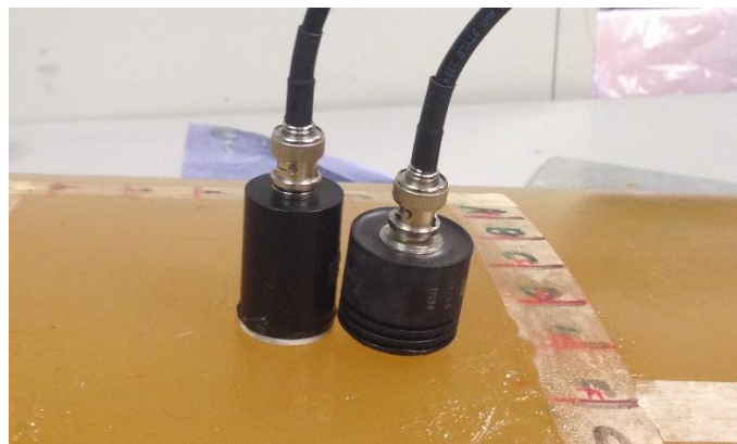
Figure 5.5: Photograph of the narrow bandwidth conventional piezoelectric transducer (right) and the, broad bandwidth piezocomposite transducer (left)
