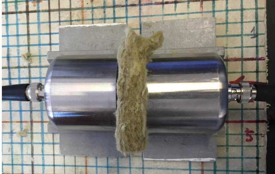
Figure 7.3: A 22 mm fiberglass wool sample under test as it dried, after being submerged in water.
