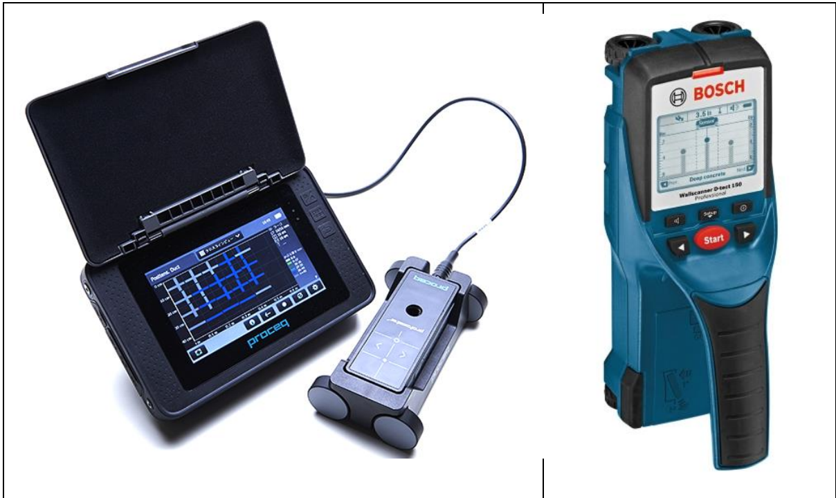
Figure 6.2: (a) Concrete cover meter [11]; (b) rebar detector [12]
