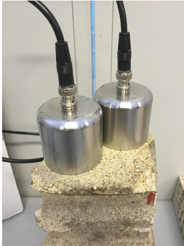
Figure 6.25: Photograph of a pair of piezocomposite transducers at the surface of a brick sample for pulse compression testing.
