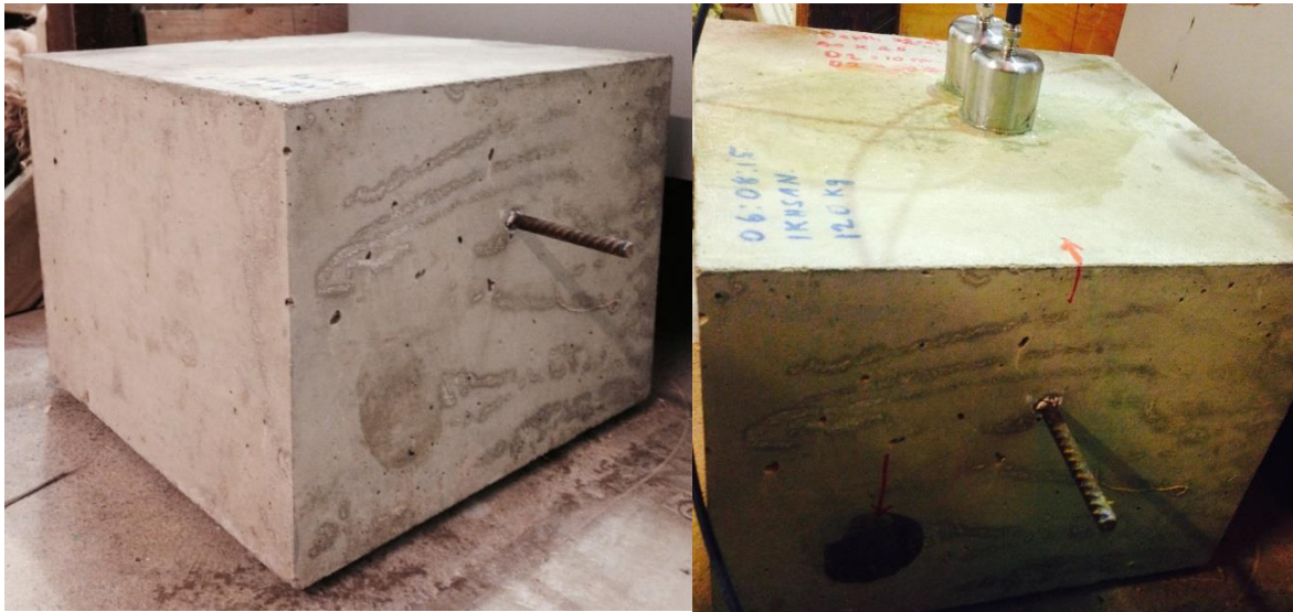
Figure 6.22: A larger concrete sample containing a rebar.
