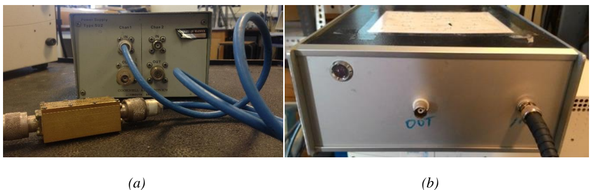
Figure 4.10: Amplifier devices available with the system; (a) dual-channel power supply type SU2 with Cooknell charge amplifier type CA6; (b) in-house fabricated amplifier
