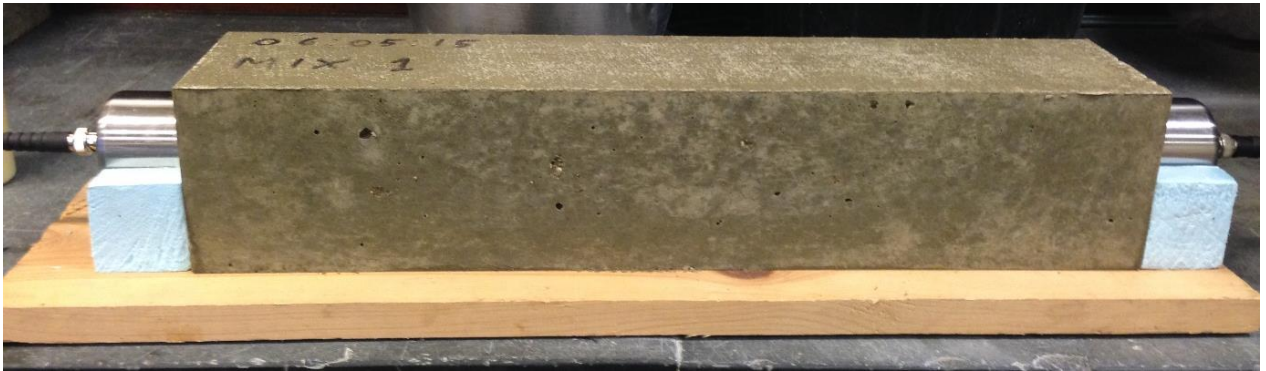
Figure 6.8: Example of concrete pillar (Mix 1) after demoulding under measurement in through transmission mode
