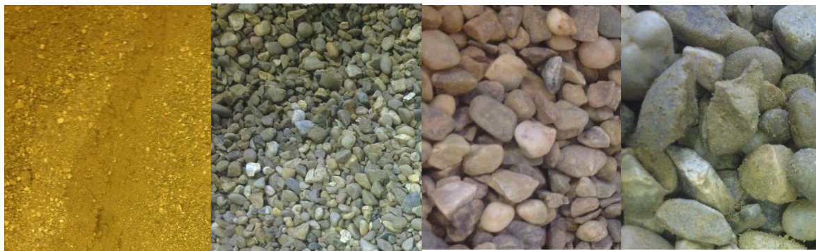
(a) (b) (c) (d) Figure 6.6: the materials used in the concrete samples; (a) sand; (b) 6 mm (max) aggregate; (c) 10 mm (max) aggregate; (d) 16 mm (max) aggregate
