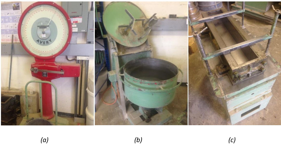
Figure 6.5: Equipment for concrete samples preparation (a) Weighing system; (b) Concrete mixer; (c) Concrete mould and vibrating table
