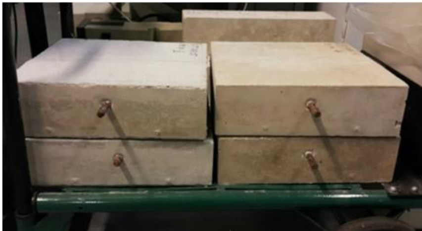
Figure 6.17: After 28 days of curing in water tank, the finished product of concrete slabs with rebar inside ready for testing
