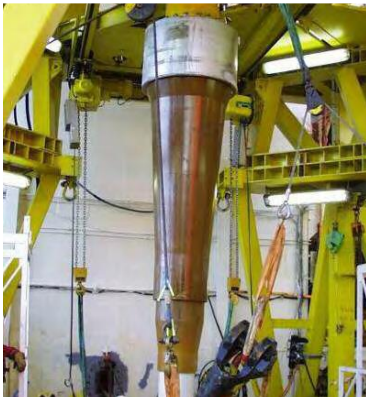
Figure 5.3: (a) Polyurethane bend stiffener as used in the oil and gas industry by Trelleborg Ltd [9];(b) BP bend stiffeners for use in North Sea oils and gas platforms [10]
