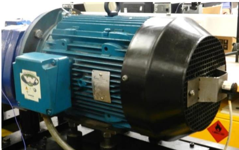
Figure 5.3 Three-phase 11 kW brook crompton induction motor
