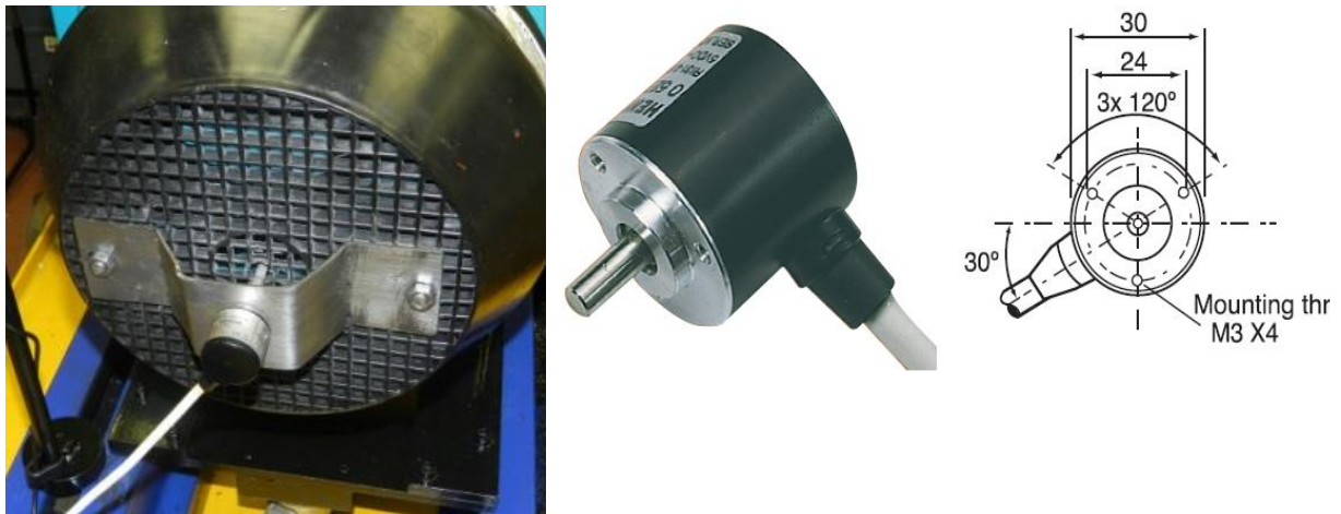
Figure 5.13 Hengstler RI32-0/100ER shaft reproduced from (Rohs 2014)
