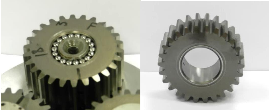
Figure 5.7 Planet gear with loose needle bearing
