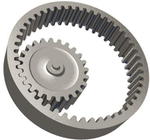
(b) Internal spur gear reproduced from (Industries 2015)
