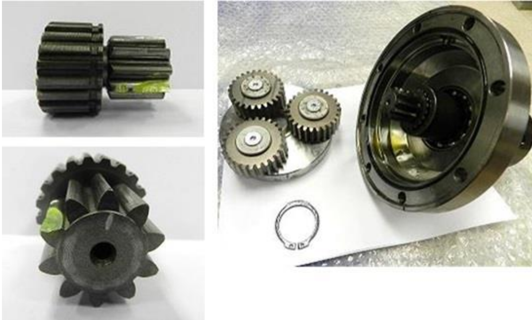
Figure 7.5 Sun gear tooth fault F2
