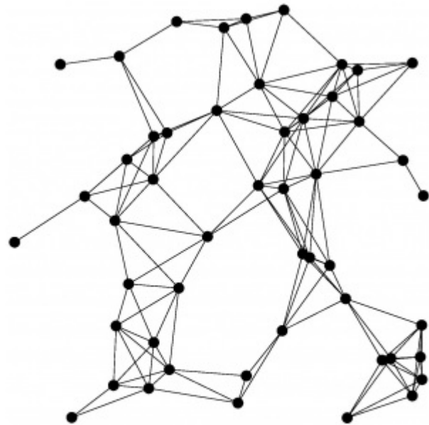
Figure 2. The vertices are wireless transceivers, with edges between transceivers which are close enough to communicate
