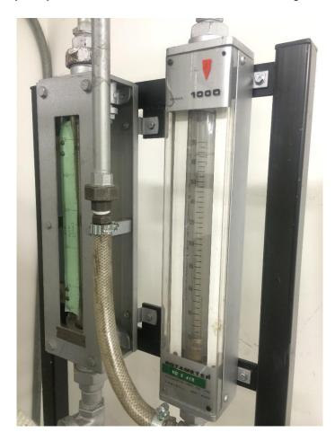
Figure 5.5: Picture of the primary and secondary rotameters used for the experiment.
