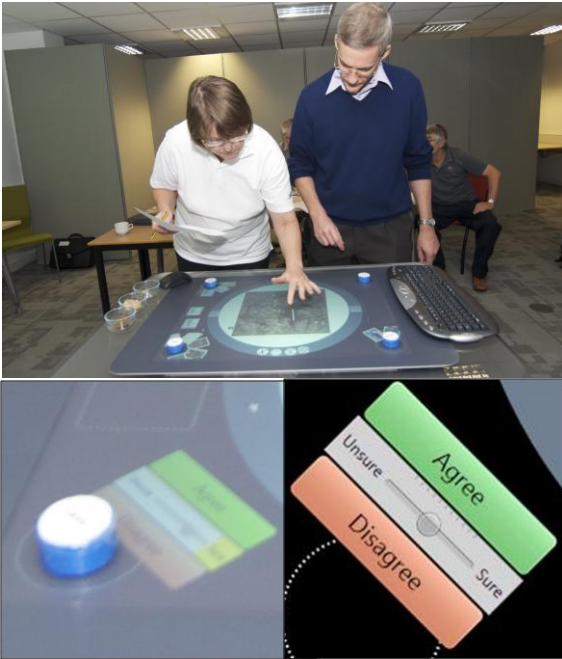
Figure 3: Tabletop computer being used for discussion of incoming images (above) and voting interface using personal tokens (below).
