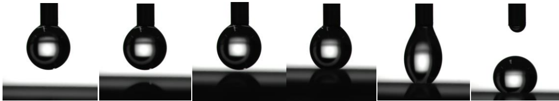
Figure 8. The process of placing the distilled water droplet
