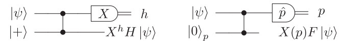
FIG. 2. Left: Hadamard gadget in a postselected IQP circuit, where h takes value 0 if +1 is measured, while h = 1 if the result is -1 . Right: Ideal Fourier gadget in CVs, exact translation of the Hadamard gadget. |0\rangle_p represents an infinitely \hat{p} -squeezed state with \sigma = 0 , thus, satisfying \hat{p}|0\rangle_p = 0 .
