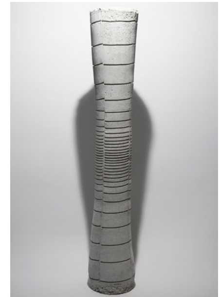
Figure 7. Waisted Column. Manufacturing process, from casting to removing the fabric formwork. Photo: Cristina Nan and Charlie Patterson.
