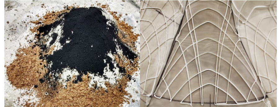
Figure 12. Material mixture for fabric cast cone. Black powder pigment was added to the aggregate, sand and cement mixture. Photo: Cristina Nan.
