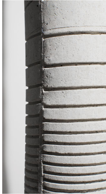
Figure 6. Waisted Column. Manufacturing process, from casting to removing the fabric formwork. Photo: Cristina Nan and Charlie Patterson.
