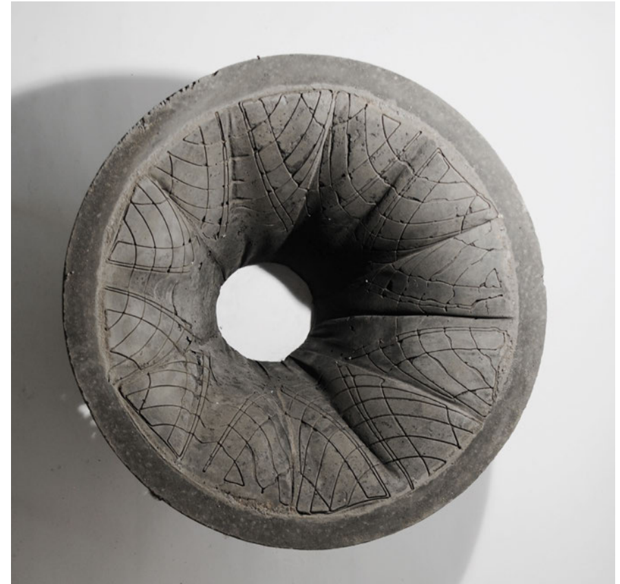
Figure 13. Fabric cast cone. Photo: Charlie Patterson.
