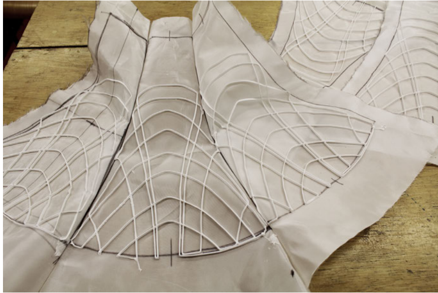
Figure 11. Cone. Fabric formwork with 3D printed patterning, partially stitched together. Photo: Cristina Nan.
