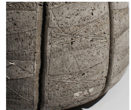
Figure 8. Twisted Column. Manufacturing process, from casting to removing the fabric formwork. Photo: Charlie Patterson.
