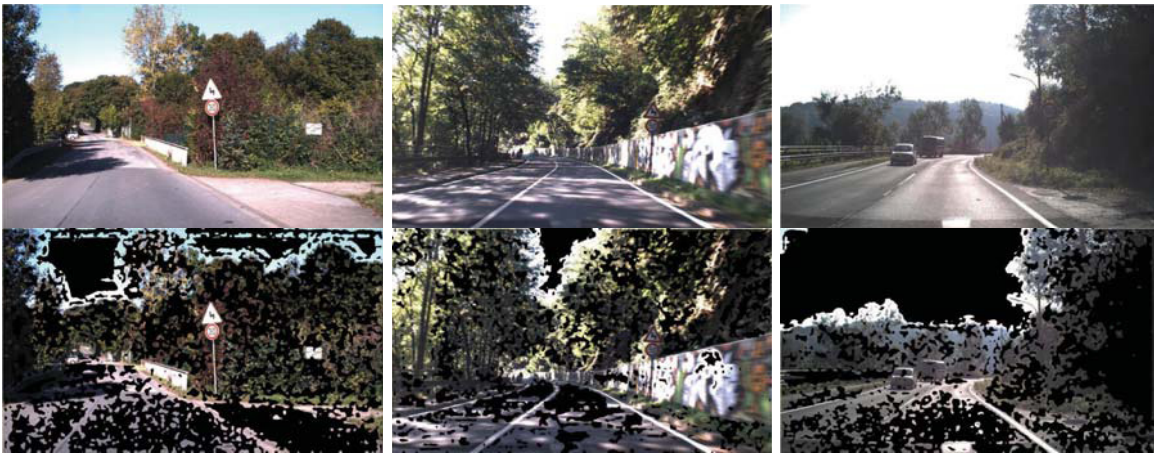
Fig. 5. Examples of saliency test. In each column, the first row shows the original image, and the second row has non-saliency pixels displayed in black.
