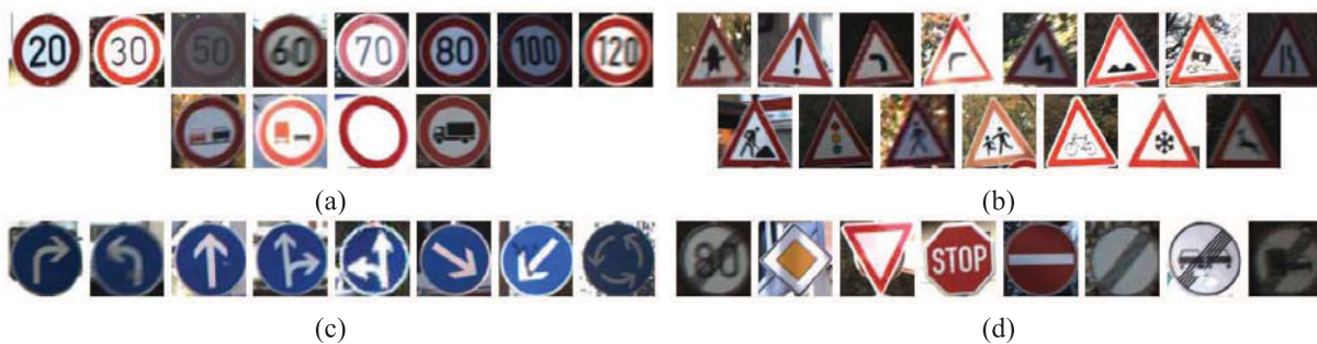
Fig. 6. Sign classes in GTSDb: (a) prohibitory, (b) danger, (c) mandatory, (d) other signs which are not evaluated in detection.
