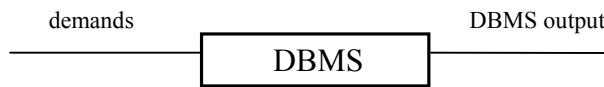
Figure 5-1. Black-box model of a DBMS. The internal structure of the component is unknown. Only its output (success or failure) is recorded on each demand and used in the inference of DBMS's pdf .
