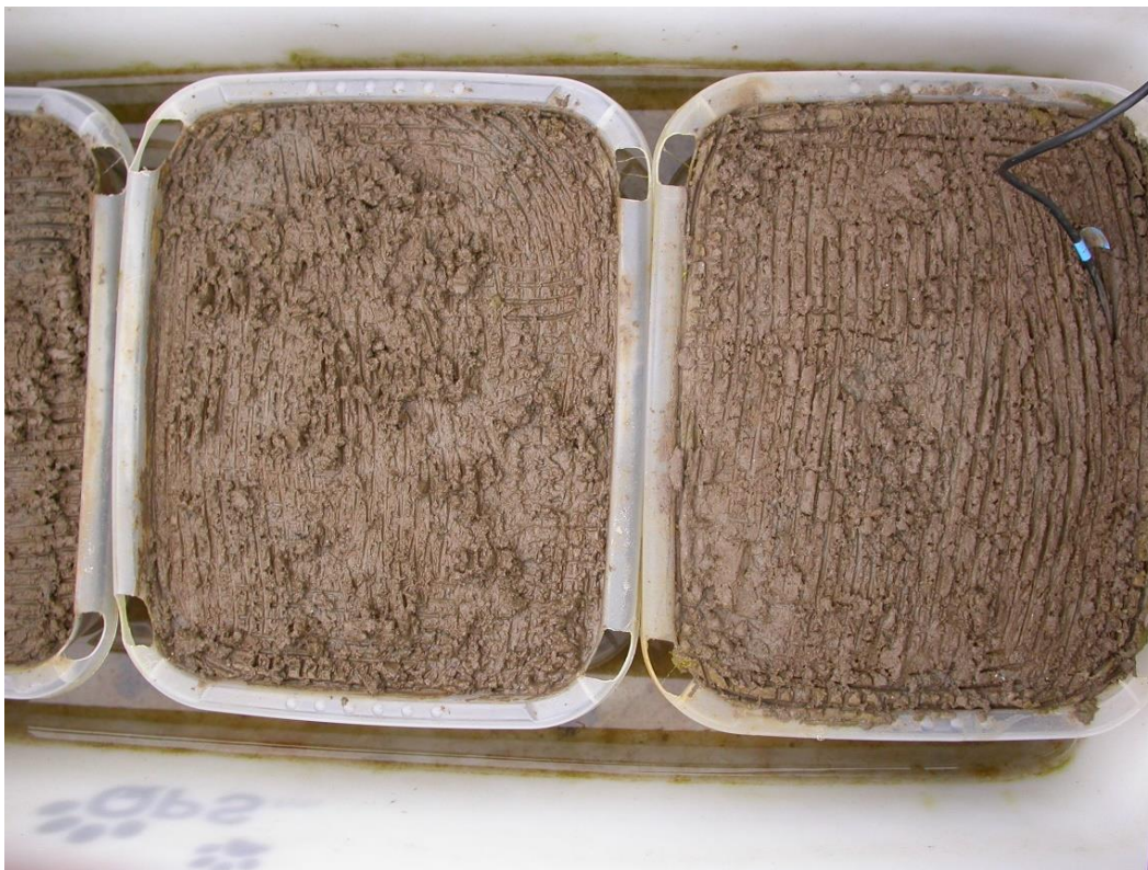
Figure 4.13. Disturbance of sediment surface (with temperature probe inserted in sediment surface of right-hand tray)
