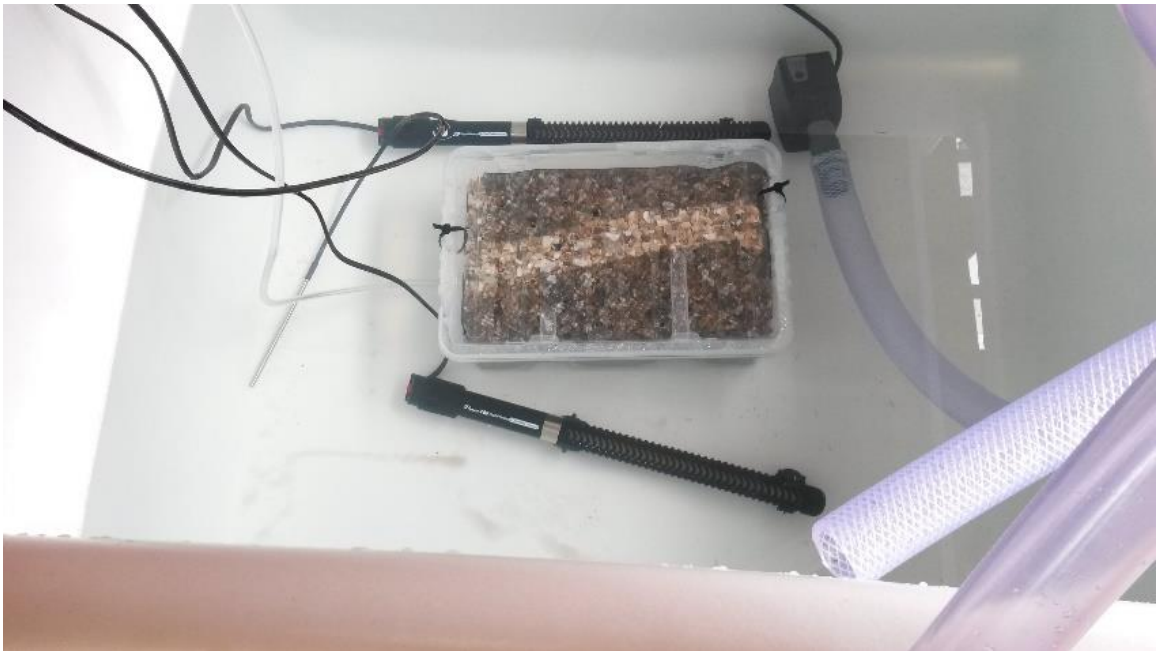
Figure 4.6. Inside of lower tank showing water pump, heaters and air box
