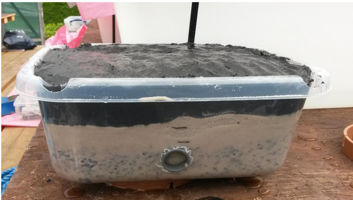
Figure 4.10. Sediment tray with layers of sand and gravel, sand and sediment
