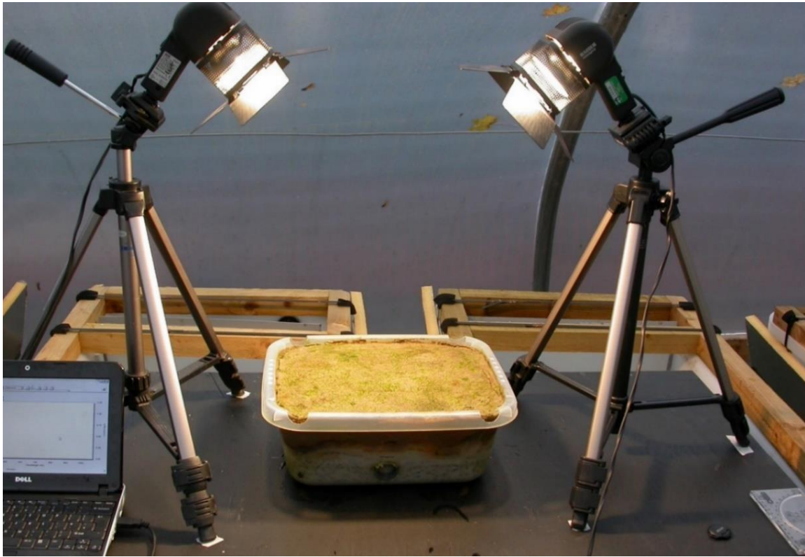
Figure 4.16. Lighting setup for reflectance measurements used to calculate NDVI and monitor biomass
