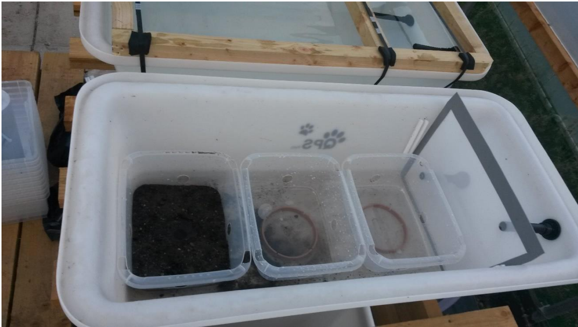
Figure 4.8. Sediment trays in upper tank showing stanchions and drainage holes
