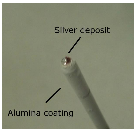
Figure 6.4-5 Silver deposit on a tungsten flat-disc electrode. Plating potential: -900 mV vs tungsten, at the temperature of 900 °C from an 1wt% AgCl in NaCl mixture. WE: tungsten, CE: graphite, QRE: tungsten.
