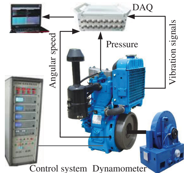
Figure 12. A photograph of the diesel engine test rig.
