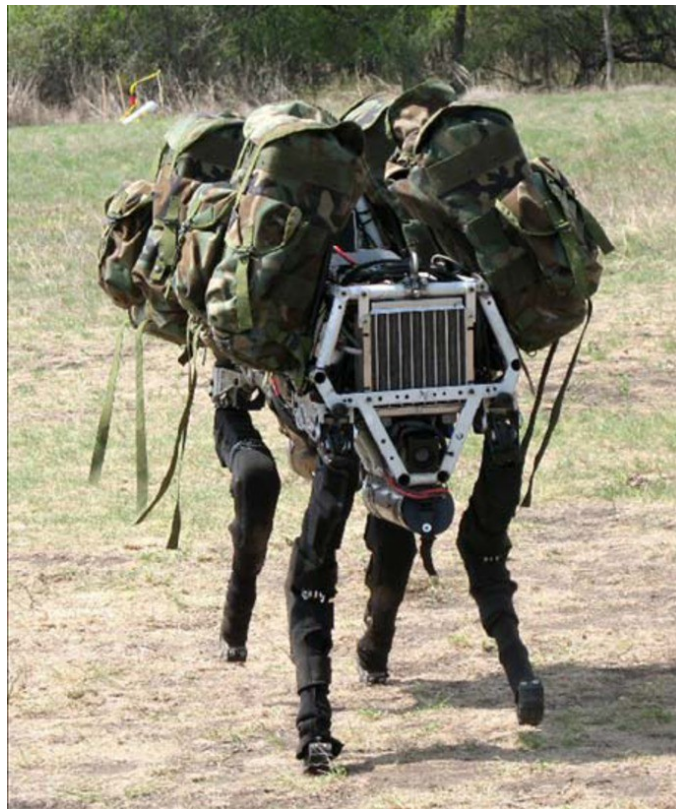
Figure 3: BigDog quadruped robot, developed by Boston Dynamics with funding from DARPA 3
