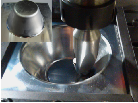
Fig. 6. Forming a part with wall angle of 70°.
