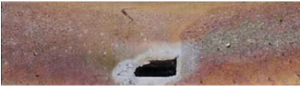
Fig. 12. Tunnel defect in cross-section morphology of an AA6061/AlN/10p joint welded at 1200 rpm and 85 mm/min [41].
